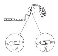
1. When you connect LED light with the LED control, please make sure the plugs remain arrow to arrow
