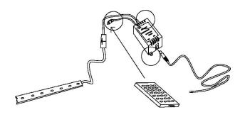
3.Remote controller should be aim at the black receiver unit when you swith colours, you can also fix the control box on the nearby wall with 2 screws, for more convenient using
