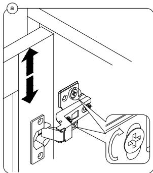
EN To adjust the door vertically loosen the screw as shown and move up and down as needed.
