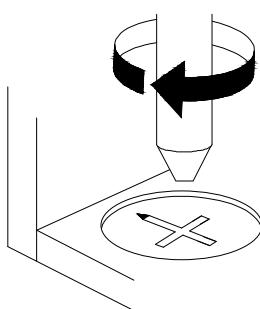
**EN** Turn cam lock clockwise to tighten.
