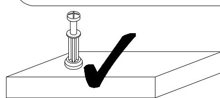
**EN QUICKFIT:** Tighten quickfit until shoulder is flush with panel. Do not overtighten or undertighten.
