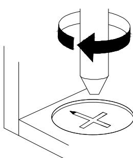
**EN Turn cam lock clockwise to tighten.**
