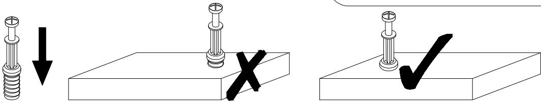
**EN QUICKFIT:** Tighten quickfit until shoulder is flush with panel. Do not overtighten or undertighten.
