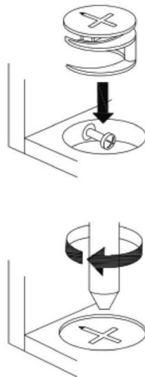
**EN\_Quickfit head** should be in the centre of the cam lock when the two panels are joined.
