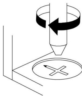
**EN\_Turn cam lock clockwise to tighten.**
