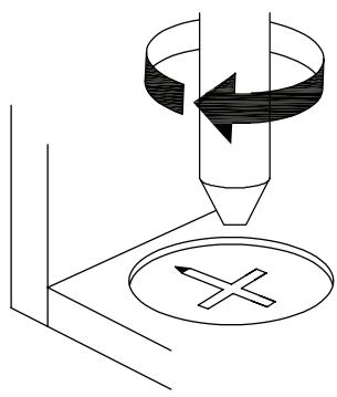
**EN** Turn cam lock clockwise to tighten.
