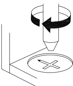
**EN**\_Turn cam lock clockwise to tighten.
